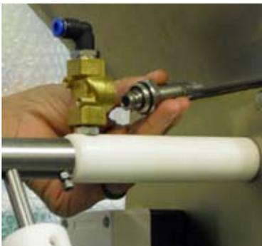
Fig. 3. Cleaning solenoid valve.
