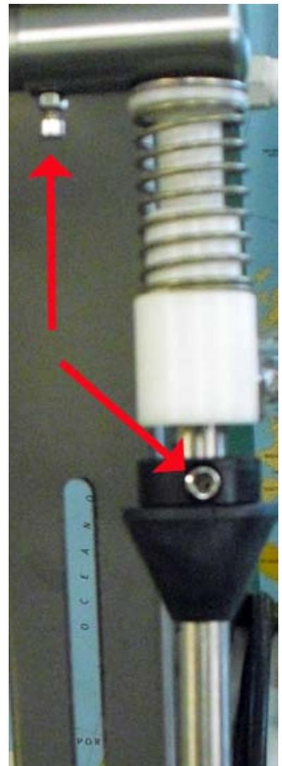
Figure 2. Do NOT overtighten these bolts.
