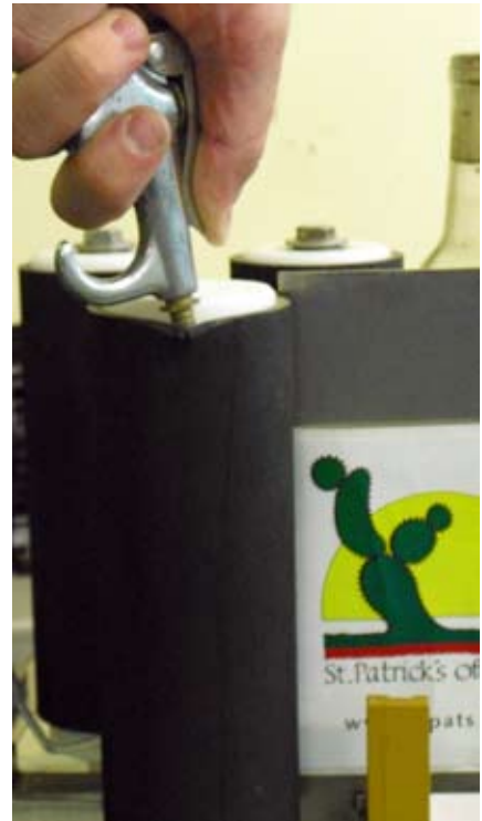
Fig. 2. Use compressed air to reposition black sleeve.
