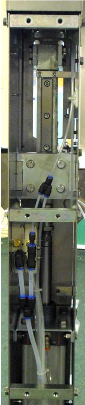
Fig. 6. Back of corker. Lubricate rail annually.
