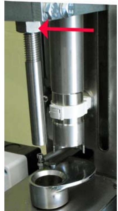
Fig. 4. Adjust Cork Pushing Pin to change depth of cork in bottle. ONLY MAKE THIS ADJUSTMENT AFTER BOTTLE HEIGHT ADJUSTMENT.
