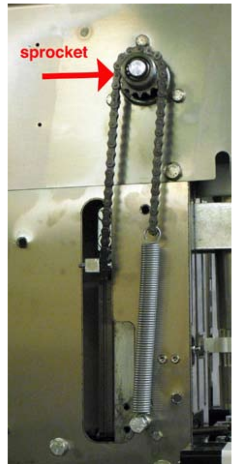
Fig. 7. Assembly to drive the hopper shaft.
