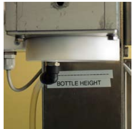
Fig. 1. Bottle Height---Top of bottle MUST be at this height or slightly higher.
